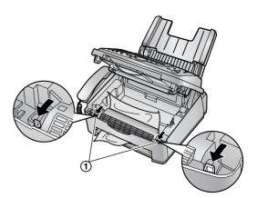
4. Remove the jammed paper (①) from the fuser unit by pulling it upwards carefully, then install the drum and toner unit.
